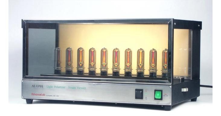
A standard model holds 10 piece of Preforms for 16 ounce or 600 ml Bottles. Other configurations and fixture sizes are specified at time of ordering More or less fixtures in a single inspection pass depending on size of Preforms
